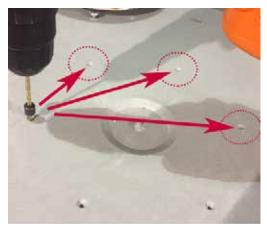
The position of the 6 holes for the screws of the k-plate is clearly marked under the table top. The collar on the drill bit should be set at **10mm** (**3/8**") from the tip of the bit.
