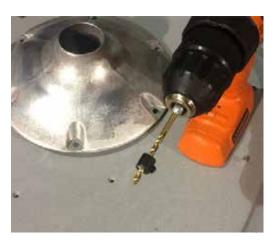
Use a **Ø3mm** (1/8") drill bit with a **collar** set to make a **pre-hole 10mm** (3/8") deep for the 6 screws holding the k-plate.
