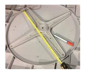
Referencing your existing plate/spider, locate the position of the screws under the new table top. We can assist and take care of this process if provided with a drawing with the interaxis of the holes.
