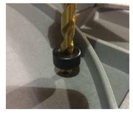
Use a Ø8mm (5/16") drill bit with a collar set to make a pre-hole 10mm (3/8") deep.
